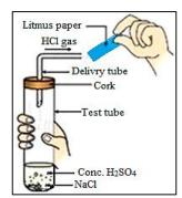
Blue litmus paper is brought near the mouth of the delivery tube to check the presence of HCI acid, but no change is observed in the colour of litmus paper because:
